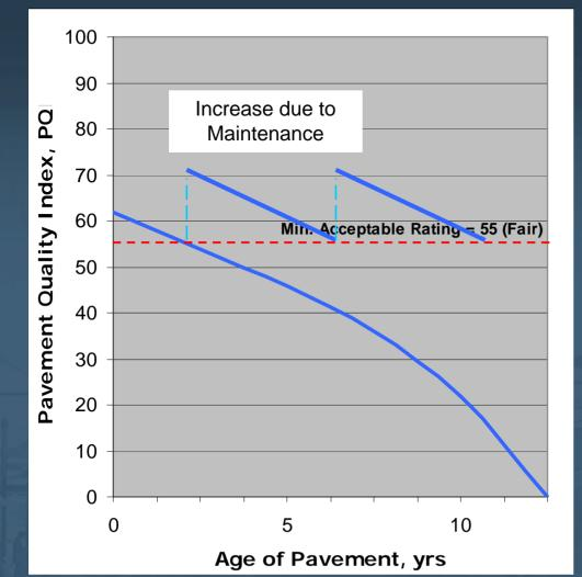
Roads with a current rating of "fair" will need a micro seal or a rehabilitation in approximately two and/or six years (870 out of 4900 lane miles)
