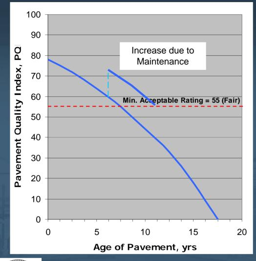
Roads with a current rating of "good" will need a micro seal in approximately six years (1484 out of 4900 lane miles)
